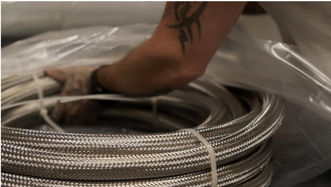
Mass spectrometer tested Clean ID assembly being bagged in preparation for shipment.
