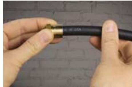
2 Insert Hose completely into ferrule and make note of how deep the hose goes.
