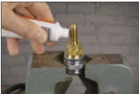
5 Add a bit of lubricant to the reusable hose barb before inserting into the ferrule.
