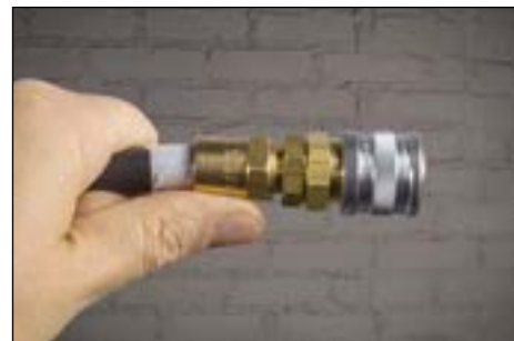
8 Completed connection, Use marker applied in step [3] to ensure hose is completely inserted.
