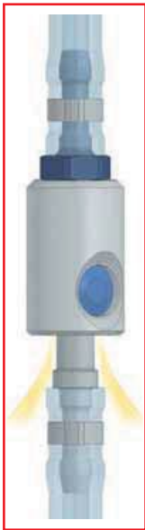
The plug is retained in the socket: dissipation of downstream pressure
